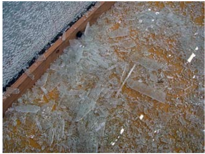
Photograph 3. Long particles remaining in the LSB impact frame after 4 mm toughened glass with surface compression 100 MPa was broken by a lead shot bag impact.
