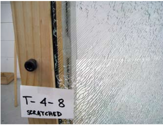
Photograph 2. Long particles resulting from lead shot bag impact of 4 mm toughened glass with surface compression 100MPa.
