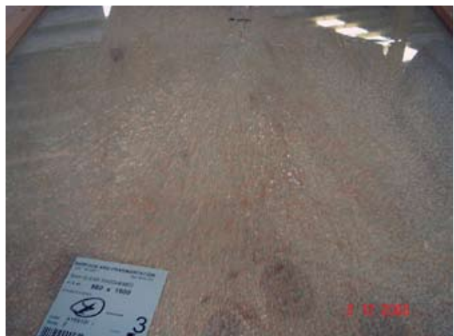
Photograph 5. This panel of 5 mm toughened glass with a surface compression of 135 MPa exhibited no long particles when fragmented at the centre break point.-
