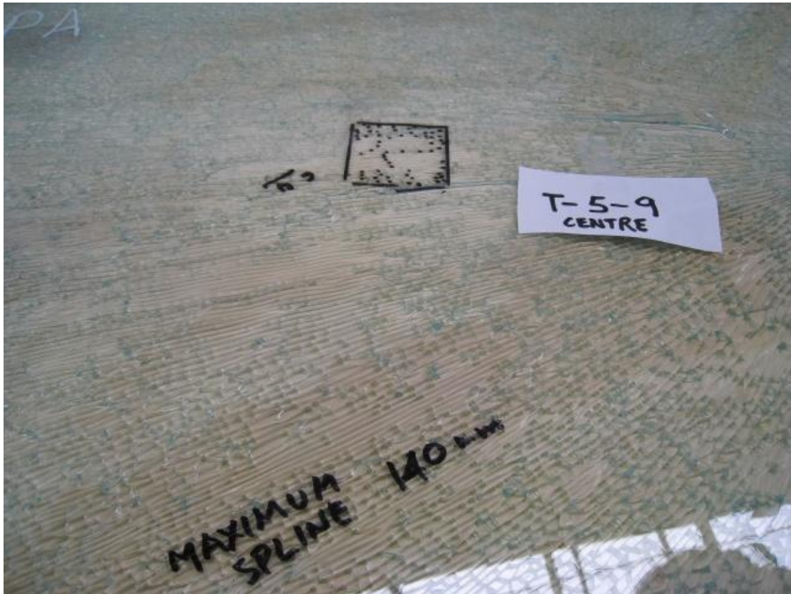
5 mm Sample No. 1_5-9; SC 114: Centre Fragmentation – Longest Particle 140 mm
