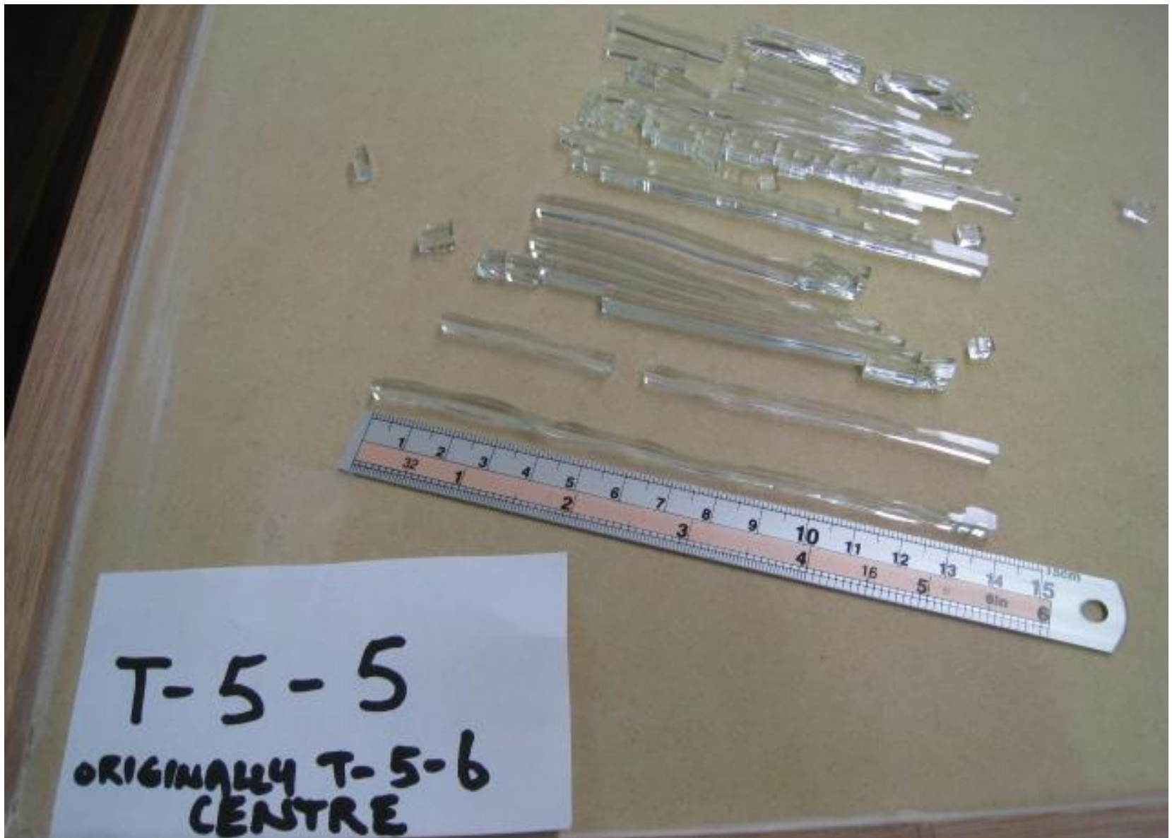
Splines from 5 mm Sample No.1_5-5; SC 107: Centre Fragmentation
