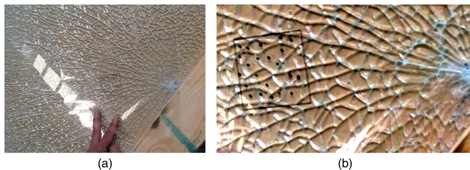
Fig. 2. (a) Test 1, 4-mm glass is broken 13 mm from the edge according to the test method in AS/NZS 2208; and (b) same image with the fragmentation count area enlarged. (Reproduced from Kidsafe 2017, with permission.)
